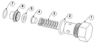
23-023 VLV, CHECK, CHECK VLV MANIFOLD
