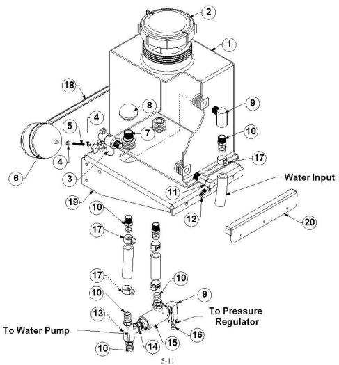
69-050 ASSY, WATER BOX THERMALWAVE II VORTEC
