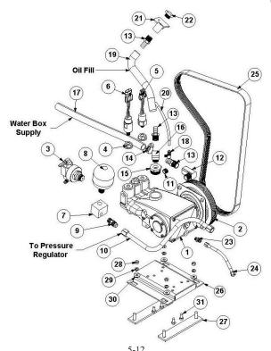
WATER PUMP ASSEMBLY TWII VORTEC
