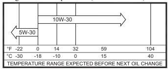
**NOTE:** Synthetic oils are not recommended for industrial or stationary engines. Gasoline engines that are converted for LPG or NG fuels MUST use oils labeled "For Gasoline Engines". Do not use oils formulated for diesel engines even when labeled heavy duty or for natural gas engines.
