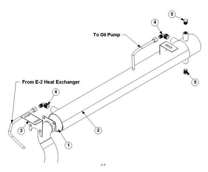
69-106 ASSY,E-3 EXHAUST HEAT EXCHANGER
