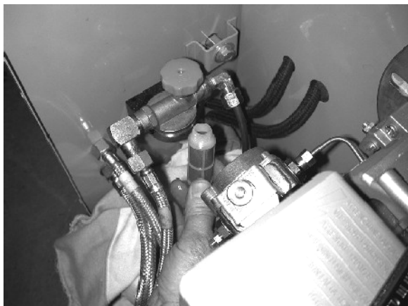
Unscrew the fuel intake filter by hand
