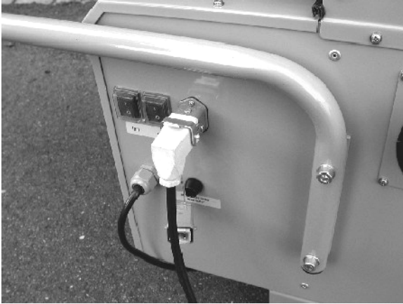
Plug the thermostat into the jack on the Dragon
