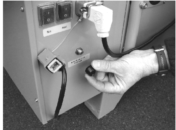
Remove the plastic cover for the Temperature-Limiter Reset Button
