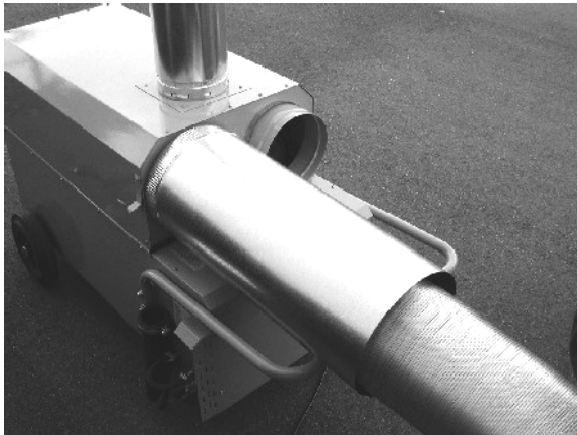
Slide the heat shields in place
