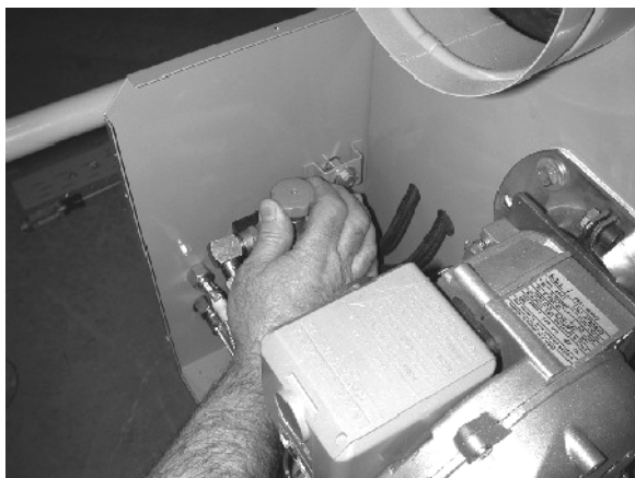
Close the fuel line shut-off valve
