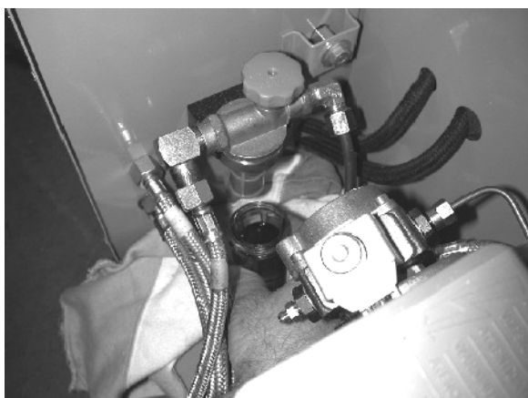
Unscrew the filter reservoir by hand
