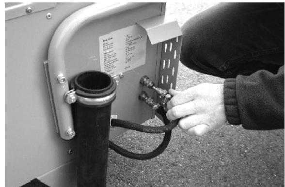
Connect the internal tank fuel lines
