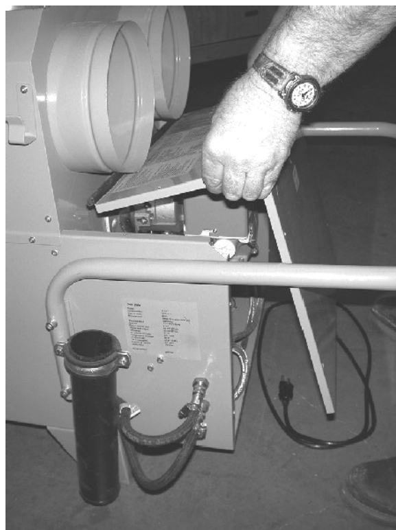
Remove the fuel pump/blower assembly housing and guard plate
