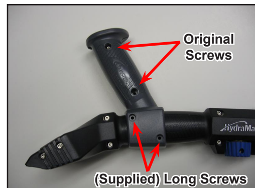
Figure 2-2. Attach Accessory Handle
