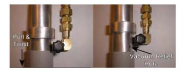
It may be necessary to periodically clean the inside of the tool, hose, and manifold. Debris can build up over time, restricting the vacuum flow.
