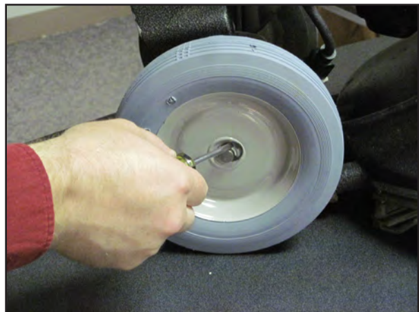
Figure 6-8. Remove Retaining Clip with Screwdriver
