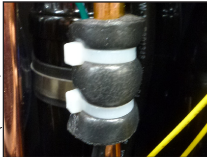
Figure 6: Thermistor attached to the refrigerant line.
