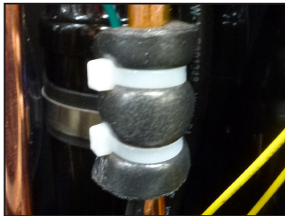
Figure 8: Thermistor attached to the refrigerant line.
