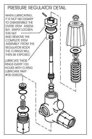
With your unit running, close the cleaning tool. Check the pressure gauge. Open the tool valve. We recommend setting the pressure regulator so that the pressure gauge reads 350 PSI with the tool valve open.
