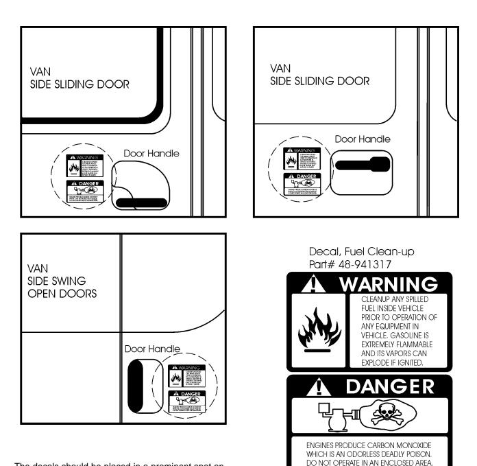
The decals should be placed in a prominent spot on the vehicle where access is given to operate the unit. The illustrations above suggest the location and placement of the decals.
