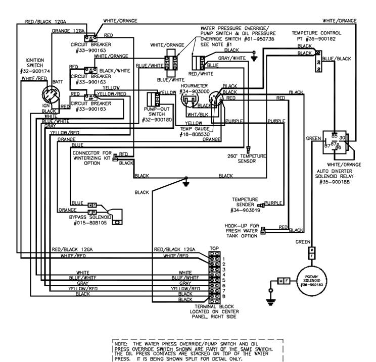
RIGHT SIDE OF SWITCH (looking at back) IS SPRING RETURN (MOM-ENTARY). "A" ON THE CONTACT BLOCK INDICATES NORMALLY OPEN.
