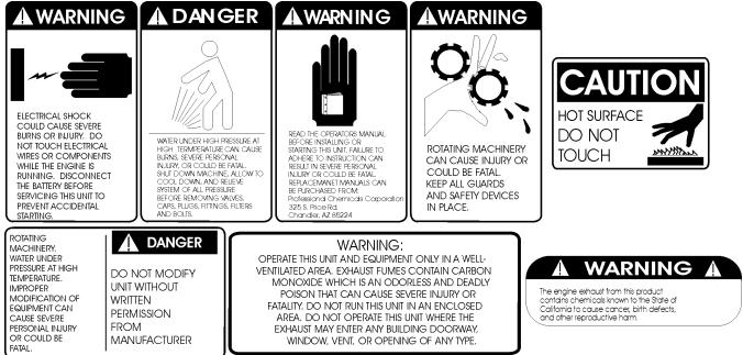
Order Part #48-941212 to get a complete set of decals (safety and instrumentation) for your *LEGEND SE* cleaning unit. The following decals must be placed in a prominent spot on the vehicle that your unit is to be installed in where access is given to operate the unit. See Figure 12 on page 3-17 for suggested locations for these decals.
