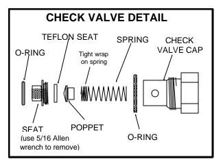
Re-assemble the check valve. Start the seat by hand, tighten using a 5/16" Allen wrench. DO NOT over-tighten seat.
