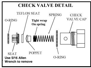
NOTE: Improper seating of the check valve poppet, damaged spring or o-rings will cause poor operation of the chemical system.
