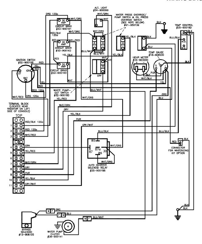
INOTE: THE WATER PRESS OVERRIDE/PUMP SWITCH AND OIL I PRESS OVERRIDE SWITCH SHOWN ARE PART OF THE SAME SWITCH. ITHE OIL PRESS CONTACTS ARE STACKED ON TOP OF THE WATER I PRESS. IT IS BEING SHOWN SPLIT FOR DETAIL ONLY.
