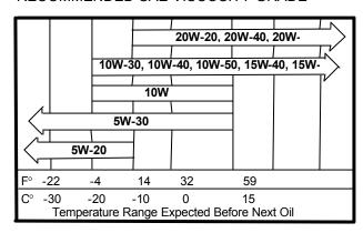
NOTE: Using less than service class SF or SG oil or extending oil change intervals longer than recommended can cause engine damage.
