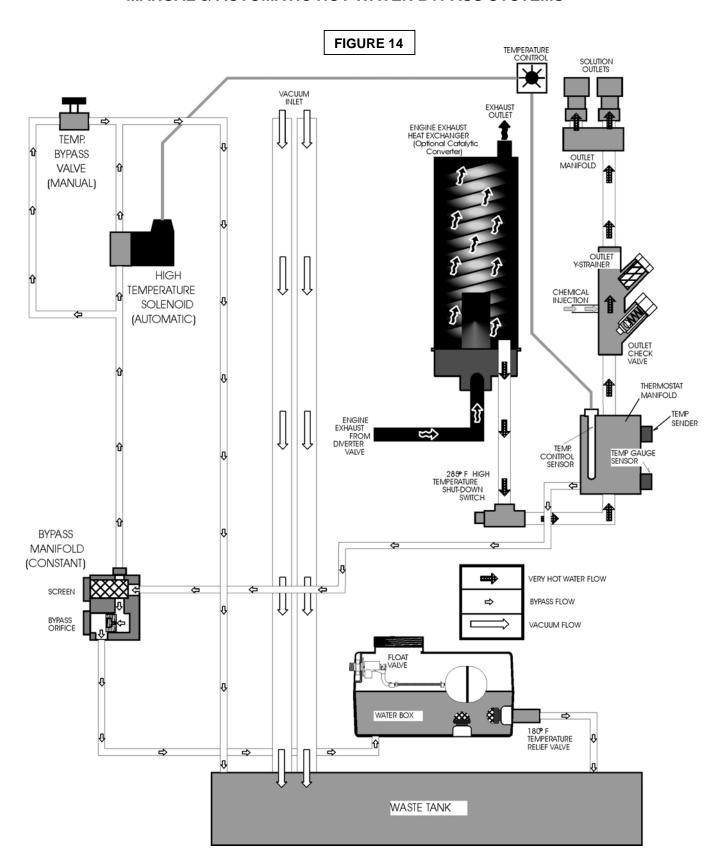
The stage three heat exchanger is an engine exhaust chamber containing a stainless steel heating coil and catalytic converter (optional). Water flows through the coil and is heated by the engine exhaust as it leaves the engine. The catalytic heat exchanger uses a catalytic core.
