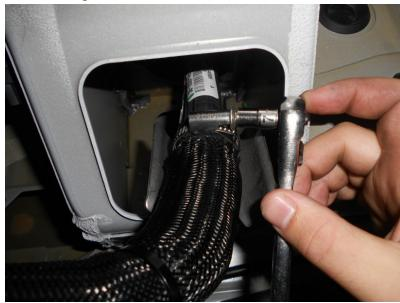
2. Remove the purge line going from the tank to the canister.
