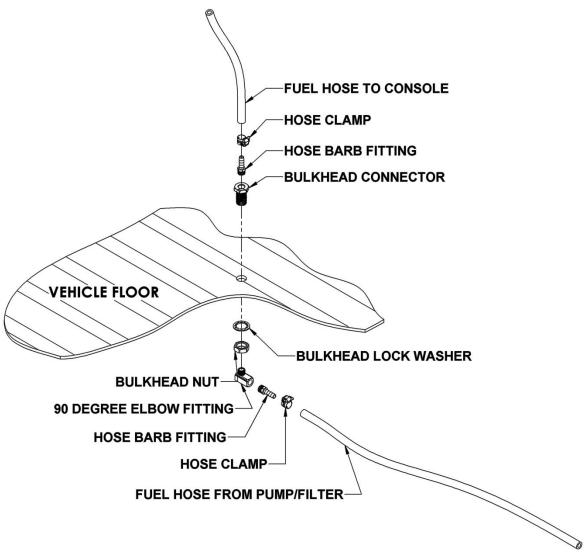
Figure 1. Fuel Line Bulkhead Assembly
