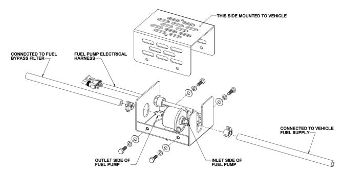
Figure 2. Fuel Pump Assembly Detail
