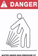
WATER UNDER HIGH PRESSURE AT HIGH TEMPERATURE CAN CAUSE BURNS, SEVERE PERSONAL INJURY, OR COULD BE FATAL. SHUT DOWN MACHINE, ALLOW TO COOL DOWN, AND RELIEVE SYSTEM OF ALL PRESSURE BEFORE REMOVING VALVES, CAPS, PLUGS, FITTING, FILTERS AND BOLTS. 44-083 /
