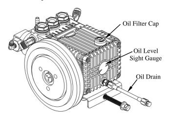
2. After the first **50 hours** of operation, change the crankcase oil with Industrial Pump Oil, (Part # 13-030). Change the crankcase oil every **500 hours** thereafter.
