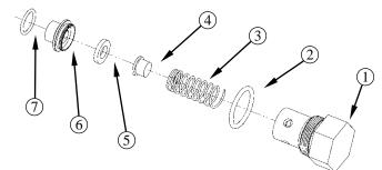
23-063 VLV, CHECK, CHECK VLV MANIFOLD
