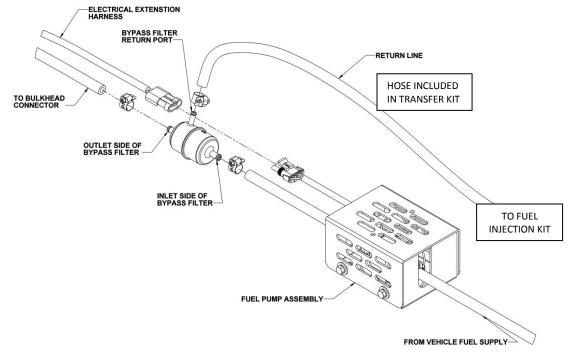
Figure 3. Fuel Pump and Filter Detail
