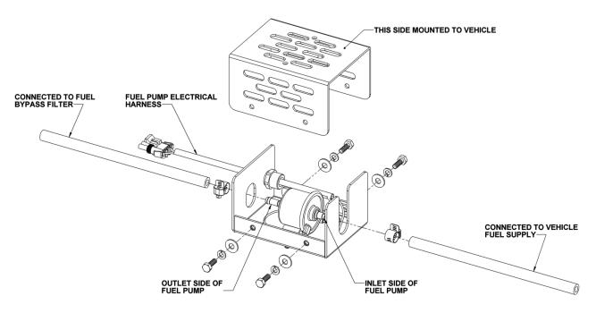
Figure 2. Fuel Pump Assembly Detail
