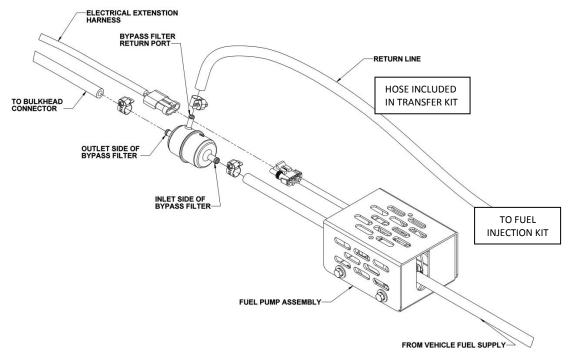
Figure 3. Fuel Pump and Filter Detail
