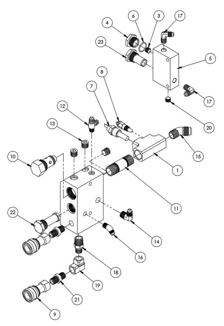
69-249, ASSY, MANIFOLD BLOCK & BYPASS MANIFOLD, 1 - 11
