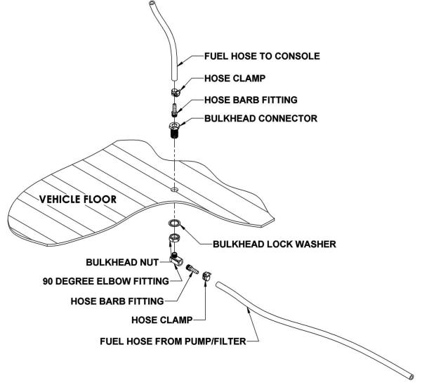
Figure 1. Fuel Line Bulkhead Assembly
