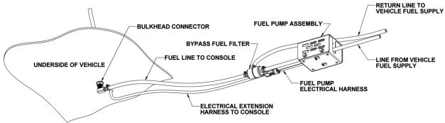
Figure 4. Vehicle Underside Fuel Line Installation
