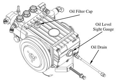
2. After the first **50 hours** of operation, change the crankcase oil Industrial Pump Oil, (Part # 13-030). Change the crankcase oil every **500 hours** thereafter.
